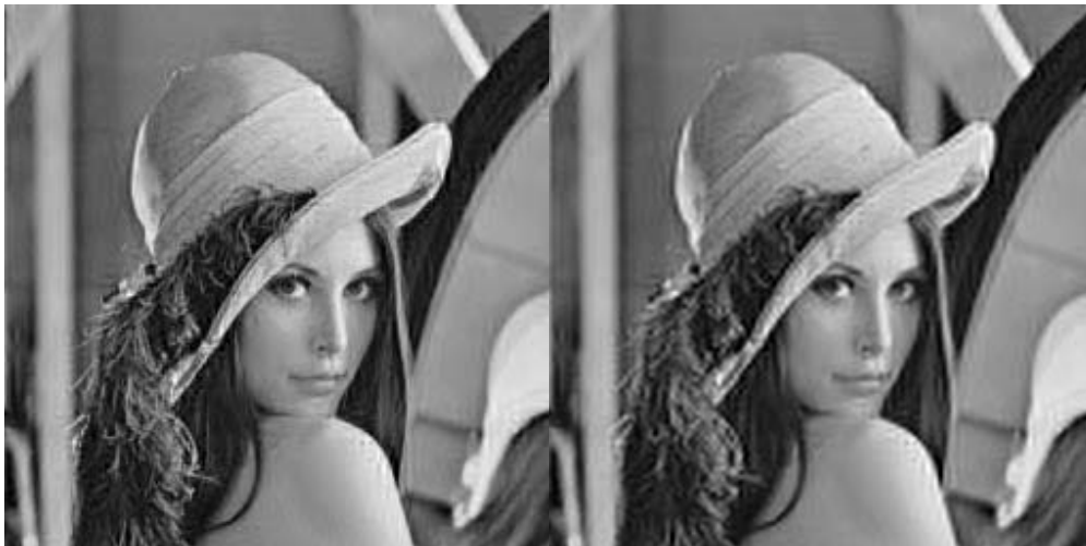
Figure 4.11: Typical compression results. The left image was compressed to 3.2:1 while the right image was compressed to 8.7:1. The maximum number of reproduction vectors for each sub-band was 256 (Figure 4.3) and no Huffman coding was used. The SNR's are 19.2 dB and 16.8 dB, respectively. Observe that quantization effects are immediately apparent as soon as a sub-band decomposition of two or more levels is used; in this example, both images exhibit these artifacts. The quantizers used were generated from the generic training set i.e., training set one.
