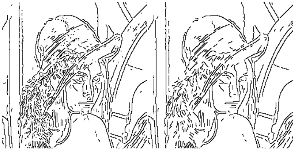
Figure 6.6: Extracted edge maps. The edge map on the left has 860 edges, while that on the right has 416. A edge length threshold was used for both — the left had all edges containing only one point removed. All edges with less than six edge points were removed from the second edge map.
