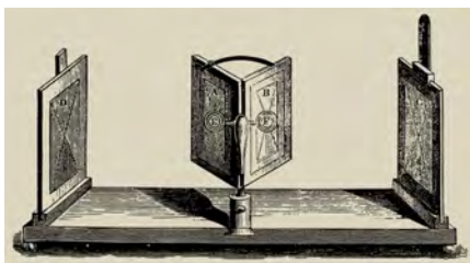
(a) The original Wheatstone stereoscope. Mirrors in the centre allowed each eye to be shown a slightly offset version of the same image (on the far left and right), simulating stereoscopic 3D. ( Wheatstone Mirror Stereoscope ).
