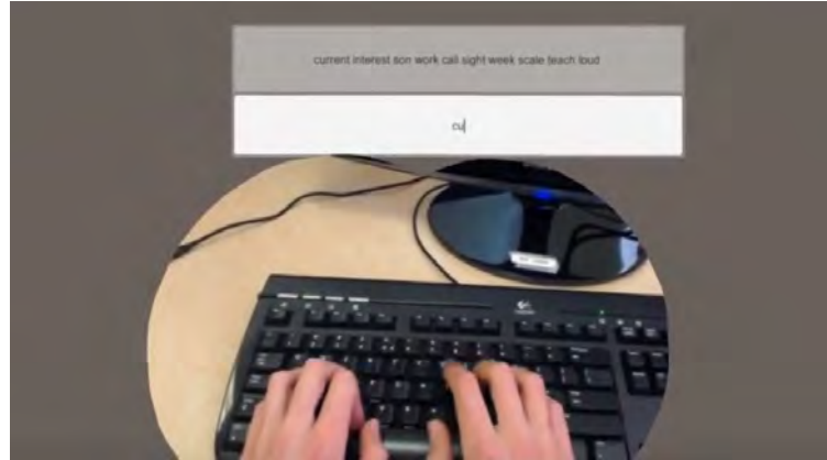
FIGURE 3.22: AV typing test. Same as the VR typing test in Figure 3.21, but with the use of the AV system enabled, allowing the user to see their hands and the keyboard while typing.
