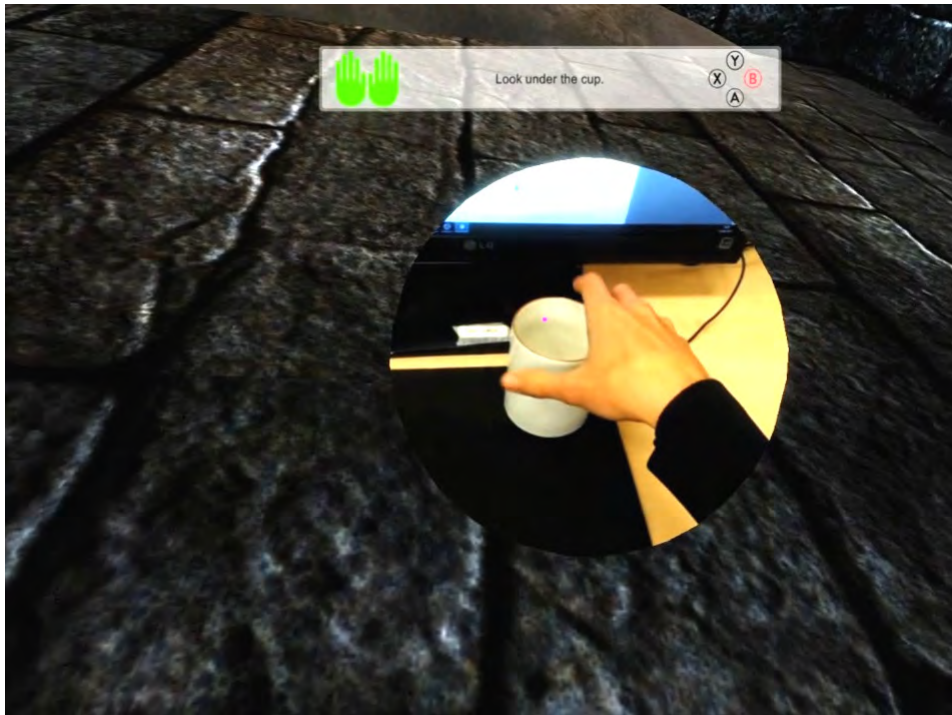
FIGURE 3.19: AV System in use. This is a screenshot from the game described in Section 3.1.2. The player has received a message in the message window telling them to 'Look under the cup'. The green icon to the left of this message indicated to the player that the instruction pertained to the real world. They have reached forward and their hand has been detected by our AV system, allowing the real world to be shown via the webcam in an area around the player's hand position. Using this window into the real world, they have managed to locate the cup.
