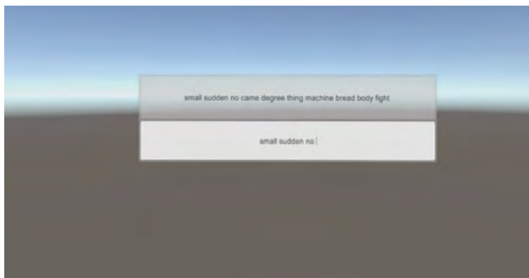
FIGURE 3.21: VR typing test. Horizon is shown in the VR version to provide visual feedback for head movement. The box containing the prescribed and transcribed text is always in the direction in which the user is looking.
