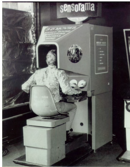
FIGURE 2.4: The Sensorama. As the text on the device indicates, the user was treated to a 3D movie, stereo sound, vibrations, aromas, and wind. ( The Sensorama Machine ).
