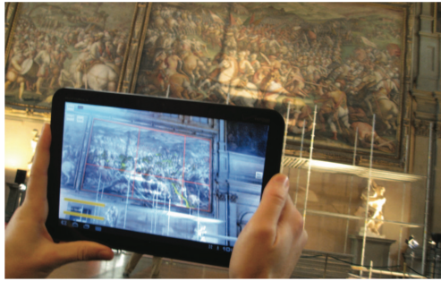
(a) The ARTifact application, a tablet-based AR tool designed for interactive analysis of cultural artefacts. Copyright©licensed content by IEEE Proceedings.
