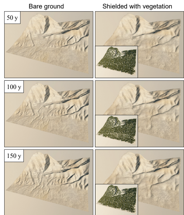
Fig. 20. Shielding effects of vegetation: a time lapse of simulations on slopes with granular materials, (left) without vegetation to damp soil erosion, and (right) protected by vegetation.
