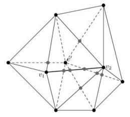
**Figure 3:** Appearance-preserving simplification, showing an edge collapse  $v_1v_2 \rightarrow v'$  in parametric space. Dashed lines represent the new neighbourhood, and dots represent the corners of cells.
