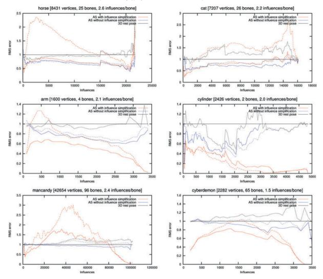
**Figure 8:** Simplification errors, normalised relative to those for 3D rest-pose simplification, for the six models. The dashed lines show standard APS, while the solid lines of corresponding colours show memoryless APS. Note that simplification proceeds right-to-left along each graph.
