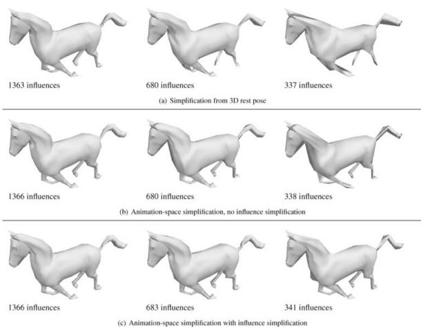
**Figure 6:** The horse at three LOD, for three simplification methods. Notice how simplification computed purely on the rest pose does not correctly handle the joints at the ankles and in the tail, causing them to vanish.
