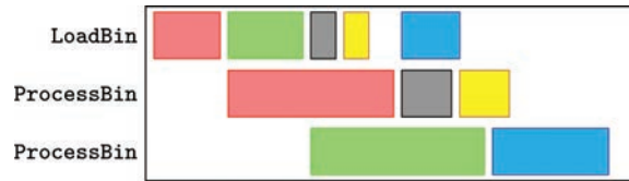
Fig. 6. Overlapping computation and sample loading. Time increases left-to-right, and each row represents a thread. Each colour represents a specific bin and shows how it is first loaded and later processed by a separate thread. The loader thread pauses before loading the blue bin so that no more than four bins are resident in memory at a time.
