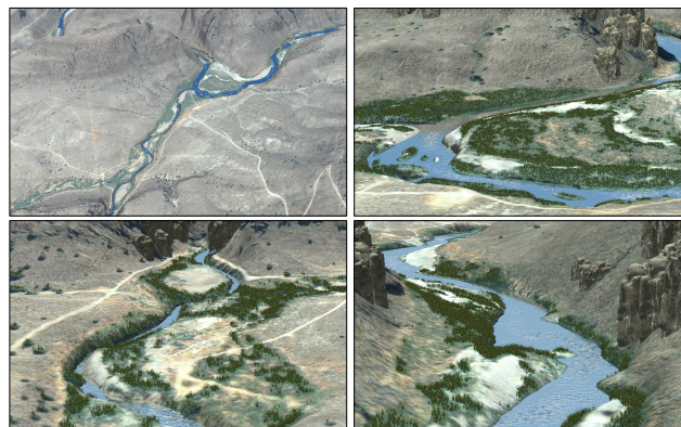
Figure 20: Real-time rendering of a river network with 698 thousands terrain and water primitives. We achieved 20–80 fps with reflected and refracted ray casting and instances of grass and rocks and 48–195 fps without these features.
