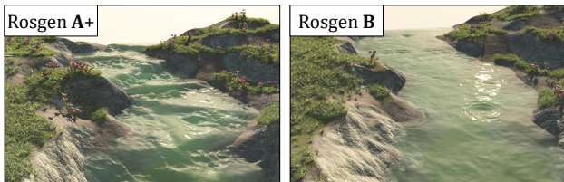
Figure 9: The influence of slope: [Left] a steep river ( s = 6\% ) of Rosgen type A+ , which gives rise to drops and basins, and matching cascades and turbulence; [Right] a flatter river ( s = 0.1\% ) with the same planar trajectory, which results in calm water primitives with a few ripples.
