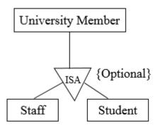
We can show both disjoint and completeness constraints in the ER diagram. Following our examples, we can combine disjoint and completeness constraints.
