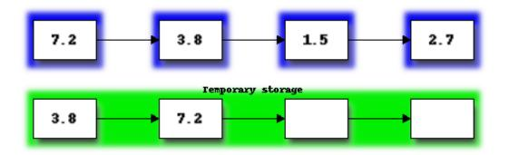
Next we copy the merged list from temporary storage, back into the portion of the list originally occupied by the merged subsections:
