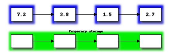
First we will merge the two sections on the left into the temporary storage. If you imagine the two sections as two sorted piles of cards, merging proceeds by repeatedly taking the smaller of the top two cards and placing it on the end of the merged list in the temporary storage. Once one of the two piles is empty, the remaining items in the other pile can just be placed on the end of the merged list:
