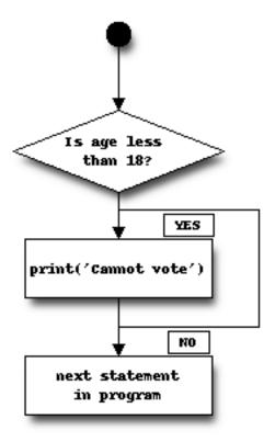
As we can see from the flowchart, the instructions in the *if* body are only executed if the condition is met (i.e. if it is true). If the condition is not met (i.e. false), the instructions in the *if* body are skipped.
